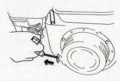
4. Pull the starter grip lightly until resistance is felt, then pull briskly.
