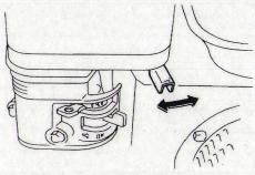
6. Position the throttle lever for the desired engine speed.
