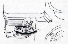
Move the GREY choke lever to the CLOSE position
