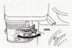
As the engine warms up, gradually move the choke lever to the OPEN position.
