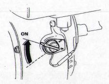
Turn the RED engine switch to the ON Position.
